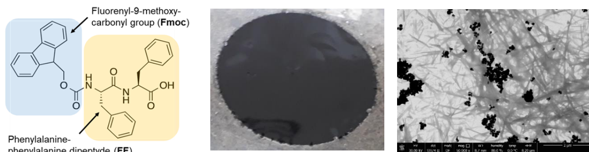
Fig. 1. Formula of Fmoc-FF molecule (left), resulting magnetic hydrogel (center), micrograph of the hydrogel structure by ESEM microscopy; the scale bar is 2 μm (right)
